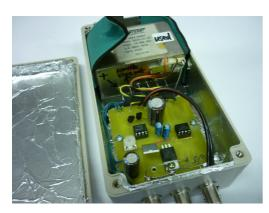
The OCXO itself is simply held in place with a cut-up mouse mat as a form of rubber shock mount. The PCB screws down on each side into the moulded plastic standoffs built into the bottom of the box.
