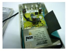
The view from the other end of the box showing the wiring to the 3 BNC sockets and the power cord (fig-8) DC wiring. The folded flap of mouse pad above the RHS of the OCXO simply exerts downward pressure on the OCXO case to keep it fixed in position.
