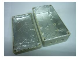
I chose to line the inside of an ABS plastic box with aluminium foil ( applied over a coat of spray glue ) because I could not readily find a suitable size diecast box - while I had the ABS box on hand.
