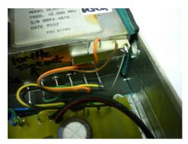
This is a close-up of the fine frequency 10 turn multi-turn trimpot and it's mounting on a tinplate z-bracket soldered to the face of the OCXO. It is accessed through a hole drilled through the side of the box. Obviously it has been moved from under the PCB.... (as seen on the PCB photos above) and contact-adhesive glued into the Z-mount.
