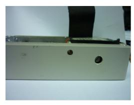
The large screw at right can be removed through it's respective hole in the side of the box and the smaller inside slotted trimmer accessed for coarse frequency adjustment - preferably with the fine trimpot near the centre of it's range - and only after the unit has stabilised.
