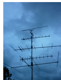
An hour later, 10:27AM, the antennas are up in the air. From the bottom : 6m yagi, 70cm vertical yagi, 2m horizontal yagi (can be "flipped" vertical), 70cm horizontal yagi, two outrigger arms - a "2m 5/8" for 6m FM and a Diamond SG-7400 for 2m FM, on top is the 23cm SSB yagi.
