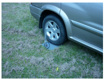
First thing to be done is to place the antenna masting mounting base under the rear wheel.
