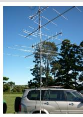
9.52AM - this view shows the red stabilising bars at the 4WD roof level. One 25mm dia tubular steel bar comes directly towards the camera and bears a 68mm u-bolt that the mast tube passes through vertically, the diagonal brace to the front bar is bolted through the rear bar and has a number of vertical holes to sit over a protruding bolt (& wingnut) fitted to the front bar. Once the diagonal brace is in position, the mast tube just doesn't move - except azumithally 'on demand'.
