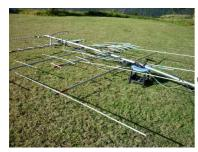
9:48AM - the antennas mostly assembled, feeders in place, white H/V polarisation change rope fitted.
