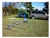
9.48AM: alternate view showing the positioning of the tilt base under the rear wheel of the 4WD - and, yes, the mast tube bends !!!! The 23cm & 70cm antennas plus the support stool and the white blow-mould table arrived in the camper trailer base - hence it still being open.
