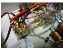
Slightly better view of the two back-to-back coax relays.
