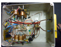
Internal view of the VK4ADC 2.4/3.4 transverter box.
