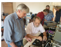
Adrian VK4OX with Doug VK4OE testing some directional couplers for return loss and coupling coefficients.
