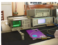
Spectrum analyser, signal generators at work, HP power meters just at the extreme right hand side.
