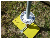
2.56PM : a view of the compass and pointer used for the grid-pack. The compass image was scanned some time ago, printed on A4, trimmed to shape and laminated onto some stiff cardboard. The wooden base is rotated until the red pointer lines up with TN then a couple of tent pegs go through the front holes to fold it in position. Rough and ready but effective.
