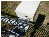
11.18AM : the 2.4 GHz transverter box attached at the back of the 24dBi grid pack. The flylead from the Conifer feed is shown terminated on an SMA male plug and screwed onto the box. The two BNC's are LO (top RHS), IF (bottom RHS) and the 5 pin DIN is used for +12V power, PTT and earth return.
