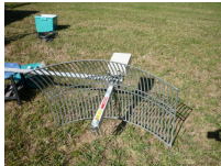
11.18AM : the 2.4 GHz physical assembly, cable form yet to be connected.
