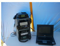
12.03PM : a quick snap of the "gear". IC-706 IF for 2.4 on the very top, the TR-751A + 23cm transverter in the middle, the IC-706MK2G for 6m, 2m, 70cm plus it's auto antenna switch at the bottom. TCXO on 10.000 MHz for both transverters (1.2 & 2.4) visible just to LHS on the table top.
