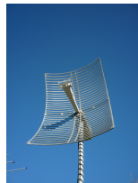
2.56PM : The modified "Conifer" feed is in use this time around. The feed should be replaced with the dual band feed for next time if the 3.4 is up and running too.
