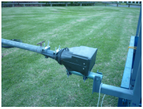
The rotator tilts outward so the masting pipe can be attached. The original hex nuts were replaced by 1/4" wingnuts to make the process simpler/quicker.
