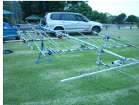
The full array of VHF and UHF antennas ready for the coax feeds to be attached.
