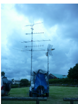
The 'weatherproofed' station. I don't like the look - or the mess - that will be fixed in version 2. Apart from the 'look', it takes to long to put up the sides even with pre-cut ropes already attached to the grommets on each tarp.
