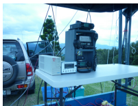
The operating table. From left, the modified UPS, the rotator controller, carry case has the 2.4/3.4 IC-706 on the very top, the TR751A plus 1296 transverter at centre, the IC-706Mk2G for 6m/2m/70cm at the bottom. This was taken before the notebook was set up to the right of the wooden transit carry case.
