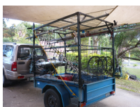
Angled view of the loaded trailer. Not much wind resistance with it set up like this. Masting pipes and VHF yagi booms up top, 70cm and 23cm yagis inside.
