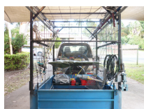
Angled view of the loaded trailer. Not much wind resistance with it set up like this. Masting pipes and VHF yagi booms up top, 70cm and 23cm yagis inside.
