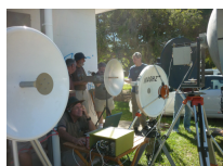
Part of the 10GHz shoot-out line-up... Adam VK4GHZ's dish set up so that his multiband feed could be tested at 10GHz.
