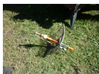
My dual-band feed and the smallest of the grid-pack reflectors. The orange conduit used to mount the feed is a tight fit into the back aluminium sleeve but allows me to adjust the feed distance.
