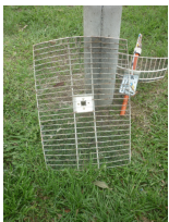
The small and mid-sized gridpacks with aluminium insect-screening attached quickly using 'liquid nails'. The W5LUA-style dual-band feed is visible on the smaller gridpack and it was swapped across during the tests.
