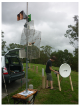
Quentin VK4AQF setting up a 10GHz dish and 5.7 GHz gear right next to me.
