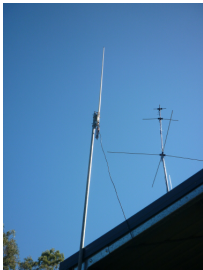
70CM homebrew collinear in foreground, top of the turnstile set in the background.
