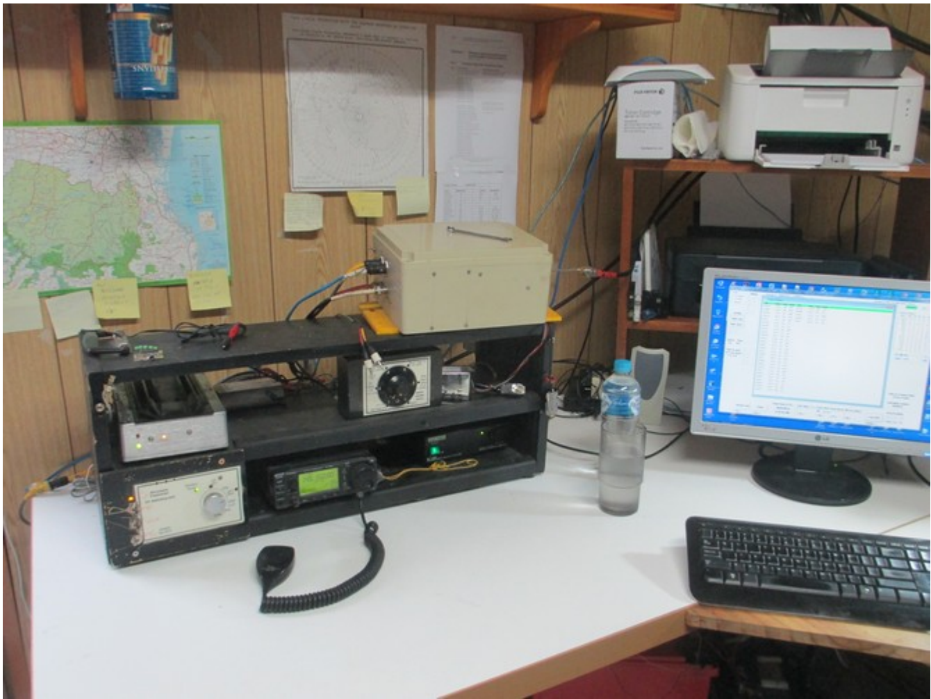
A slightly better view of the transit box with the 23cm transverter at mid-LHS plus the beige/grey 2.4/3.4 transverter box. The 'box' was powered by the small switch-mode AC supply at bottom RHS of the bottom level of the box.
