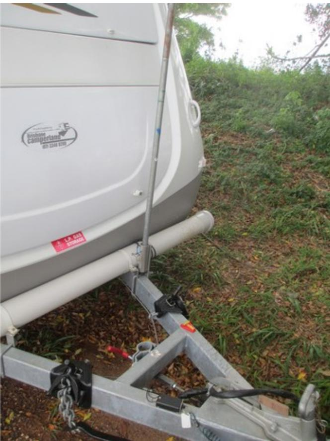
I have fitted "tube mounts" on both the front and rear of the caravan so that I can readily mount antennas like my squid pole. On this occasion, it was used to mount the pipe with the turnstile array on top.
