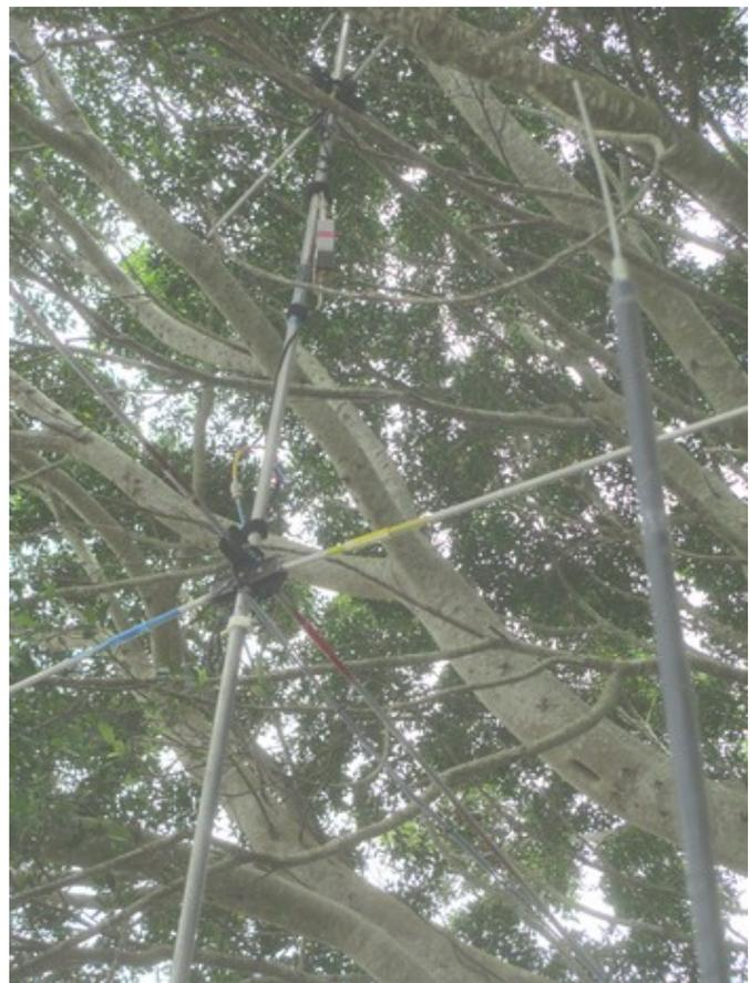
The 6M turnstile is easily seen with the 4 colours of paint to indicate which 'socket' the individual elements match up with (red/blue/yellow/maroon). The diecast box for the 2M/70CM diplexer (grey diecast box, red stripe, side on) is also visible but the 2M and 70CM turnstiles are actually hard to distinguish amongst the tree branches. The black whip at extreme RHS is a 40M Mobile One helical whip.
