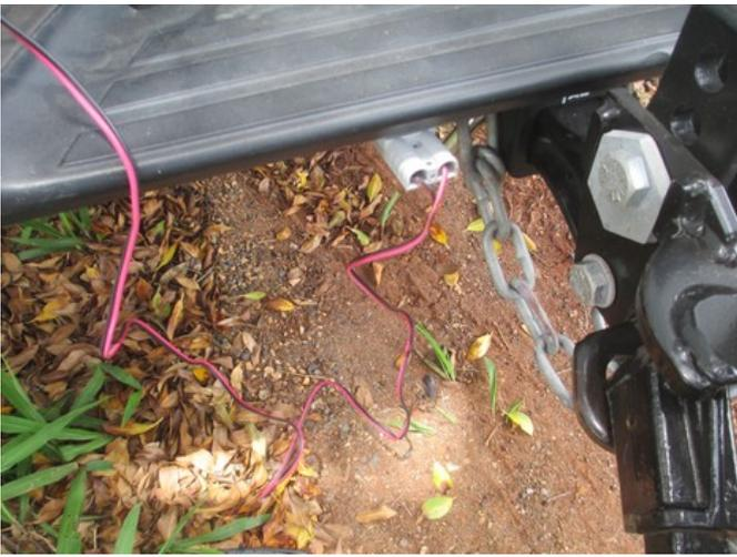
Power from the 50A anderson style socket on the back of the truck was the obvious source of power for the IC-7000.
