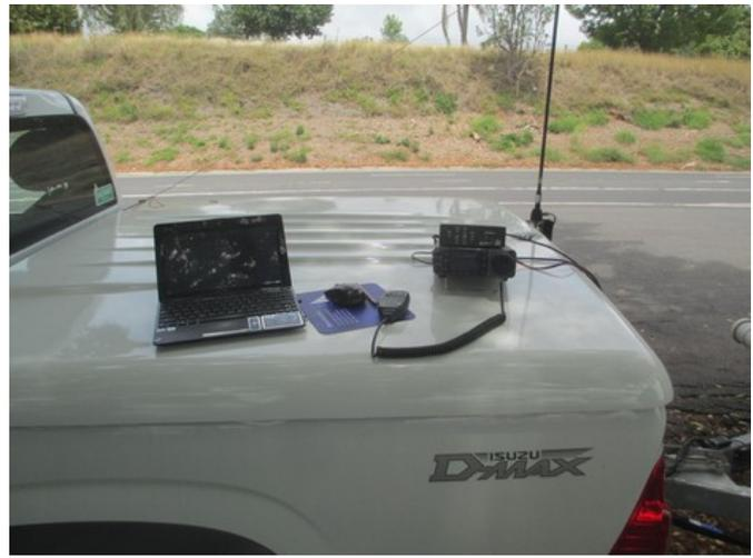
The final operating position: Icom IC-7000 with LDG tuner on top, the Asus Netbook for logging. The whip at right is a 40M helical on an L-mount.
