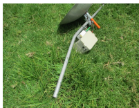
The inner section of the microwave masting after the failure of the bracket on the trailer. The bend occurred just below the 2.4/3.4 GHz transverter mount. Trying to use it would have meant that the dish and gridpack would likely be pointing at the moon.
