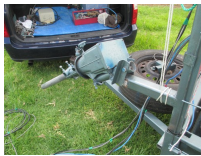
The bracket that broke off was on the LHS of the rotator mounting stub pipe. The rotator plus broken bracket was put more-or-less back in position for this photo.
