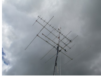
VHF/UHF antennas up vertical - phase 1. Yagis for 6m, 2m, 70cm horiz, 70cm vertical plus a 2/70 whip on the very top.
