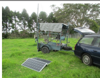
The weather was such that I only required the top cover polytarp for the event. The two 80w solar panels in the foreground helped keep the battery bank up but the overcast conditions certainly limited the available charging current.
