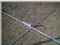
The anti-sag bracket overall view
