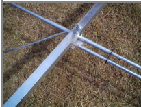
Anti-sag wire goes through the top of the DE U clamp
