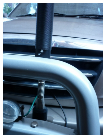
The second vehicle has a heavy duty base mounted off the inside of the "nudge" bar - but there is insufficient clearance to just screw the base loading coil onto the base itself.
