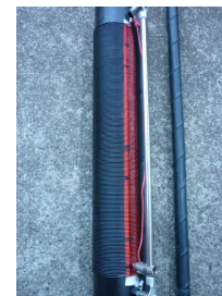
Second view with the sliding contact virtually at the bottom of the coil so minimum introduced inductance.
