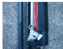
This shows the wire fully extended when the slider is at the bottom of the coil.
