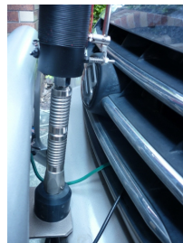
Fortunately I still had a couple of 5/16" spring bases and they provide just enough height to avoid the horizontal section of the "nudge" bar.
