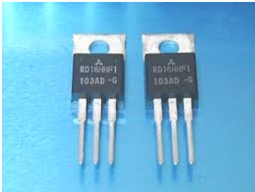
Two more "real" RD16HHF1 devices, note the Mitsubishi logo and dimples, the part number and then the batch number detail on the 3rd line.
