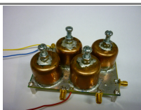
This is the top view of the completed W1GHZ transverter PCB for 2.4/3.4GHz.
