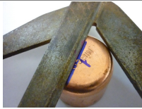
Marking out the centres with a 45 degree square
