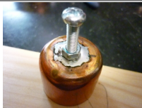
After drilling to 6mm and tinning with solder
