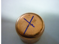
Marking out the centres with a 45 degree square
