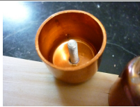
Inside view of the pipecap. This is what it will look like inside once assembled onto the PCB
