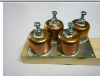
The 4 pipecaps soldered to the top of the PCB
