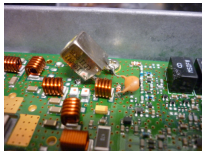
This was the first FT-1802M to be modified. The only obvious difference is that the capacitor has it's value underneath and therefore not visible and that it is at a different angle to the other unit.
