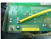
The wiring across the rear rocker switch was fed through some yellow heatshink due to it's proximity to the 240VAC generated within the UPS
