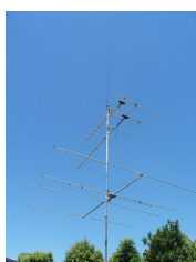
The yagis on the mast tube. This photo shows the 5/8 wave whip on the top too
