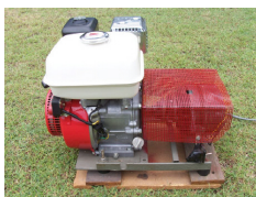
Ron VK4KLC's home-made generator using a 4 stroke 5HP Honda motor.
