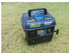
GMC generator with 240VAC available from under the protective flap on the front cover
