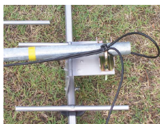
Rear view of hinge when assembled onto the mast tube
