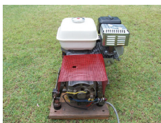
View showing the car alternator inside the safety cage
