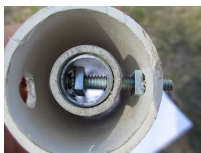
The inner tube end showing the spring washer plus internal nut.
