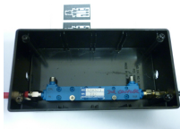
The inside of the plastic "jiffy" box. I know it should be metal but... The extra holes in the middle of each side were drilled before I realised I needed to allow space for the long-ish 2 x SMA coupler connections...
