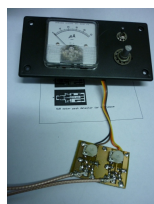
This shows how the PCB is wired across to the meter with a piece of 4-wire ribbon cable.
