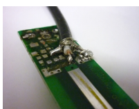
The 9006 cable soldered at the end of the balun section.
