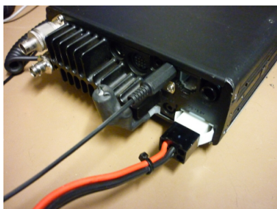
The input is derived from the CIV port on the back of the IC-706 (top black 3.5mm mono plug)
