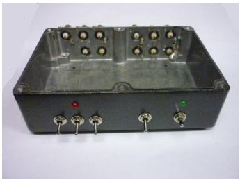
Front view with the toggle switches & LEDs mounted. Inside view of rear BNC sockets.
