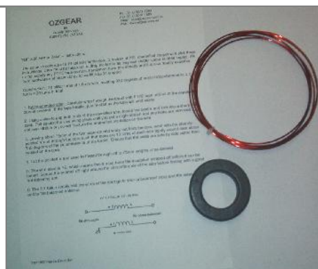
Typical kit contents TBF1000 illustrated - core, wire and instructions.
