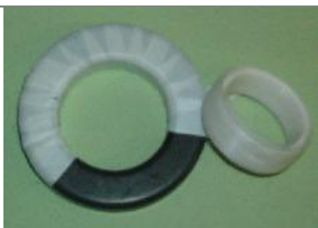
Taping core with PTFE tape FT-240-61 core used
