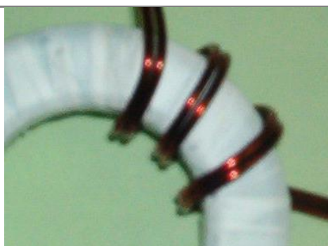
Bifilar winding technique - thread two wires "as one" - without significant gaps for the entire length of the specified turns.
