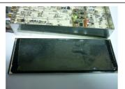
The bottom of the box is sealed off by a tightly fitting tinplate lid lined with a RF absorption foam material. To prevent inadvertent connection to the X-Locker PCB, the foam was covered by a piece of plastic packaging tape. The indentations seen towards the RHS are from where the components on the X-Locker have made physical contact.
