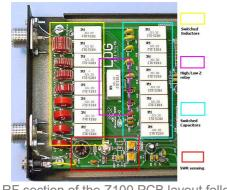
The RF section of the Z100 PCB layout follows the same trend as the Z11 image shown here. The microprocessor part of the unit has been updated to reflect the later technologies but it still does the same thing : measure the forward and reflected voltages and either sets, or re-sets, individual latching-style relays.
