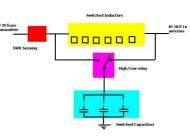
The interesting part of the schematic at left, and made more obvious by this conceptual block diagram, is the relay contacts at the upper right hand segment. This relay switches the capacitor "bank" (or switched C network) across either the input or output connection thus creating either an "L-network" impedance transformation network either up or down in ratio, i.e from 50 ohms to a higher impedance (eg 50 to 1000 ohms) or from 50 ohms down below it (i.e 3 to 50 ohms).
